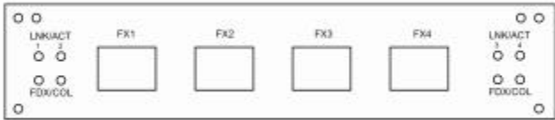
Figure 3: Illustration of FX LEDs represented by FO-065-75204VF
