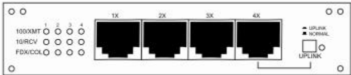
Figure 5: Illustration of Uplink function, only necessary on FO-065-75204TX
